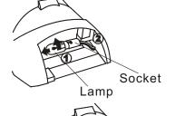
Push a new lamp gently into the socket and turn it clockwise to tighten it.
